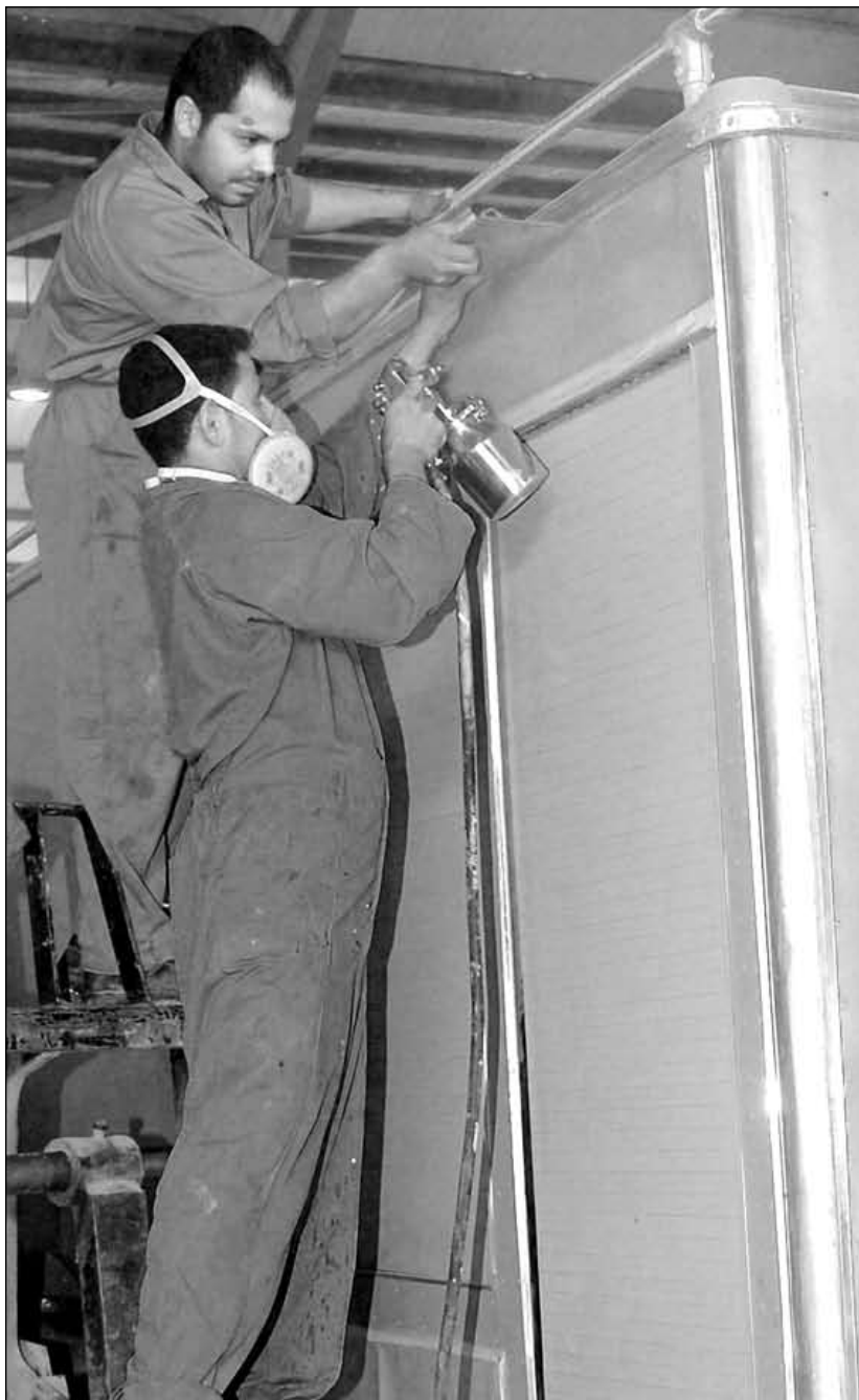
CAMP TAJI, Iraq – An Iraqi Soldier finishes a new paint job after replacing damaged body panels at the level III Maintenance facility on Camp Taji, Iraq, Sept. 27. The Level III facility is striving to repair 60 vehicles in 30 days as part of an Iraqi Army initiative to further enhance and challenge the capabilities of the Iraqi maintenance Soldiers working there.
